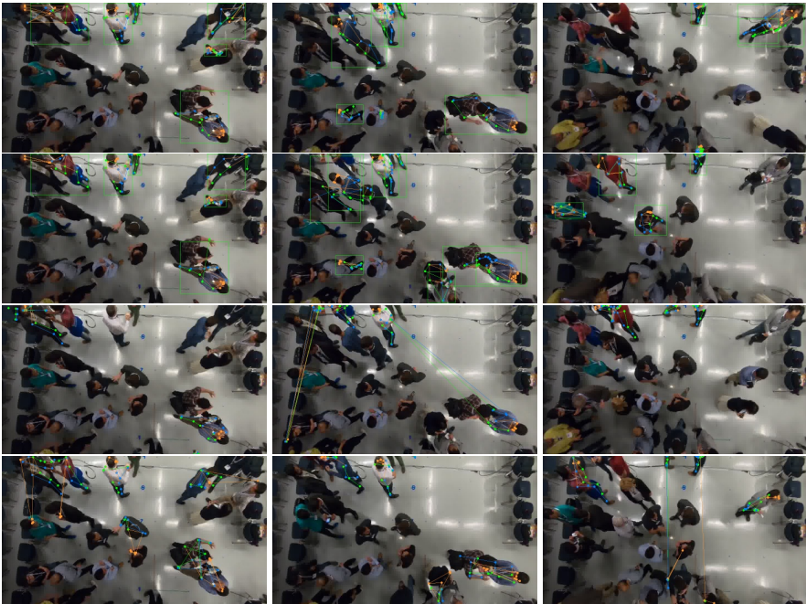
Figure 2.17: Results from Pretrained keypoint detection models. From top to bottom - predictions from RSN [28], MSPN [83], HigherHRNet [84], and HourglassAENet [85]. Results show that SOTA 2D body keypoint detection models fail to capture the body keypoints in the ConfLab dataset.
