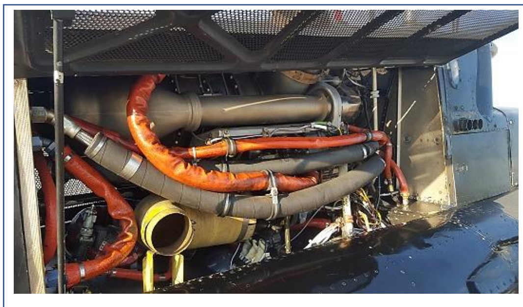
Figure C.1. The Allison T63-A-720 gas turbine engine. This photo shows the engine, as installed on the Jet Ranger helicopter.
