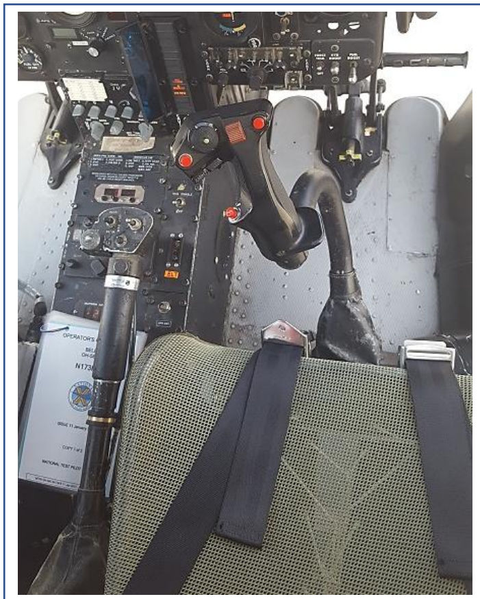
Figure C.2. The Jet-Ranger flight-controls. This photo shows the pilot seat (right-hand side) flight-controls; the cyclic-stick, the tail-rotor pedals (only the right pedals is shown) and the collective stick mounted to the left of the pilot seat.
