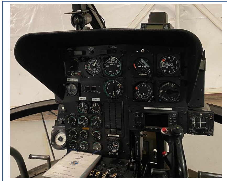
Figure C.8. The BO-105 Instrument Panel. The pneumatic flight instruments are located first from the right (pressure altitude on the top row and vertical rate of climb/descent on the bottom). The airspeed indicator is located on the top row, third from the right.
