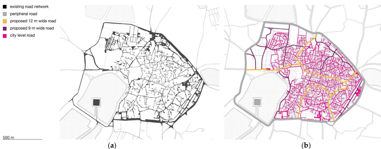
Figure 7. Town Planning Scheme (TPS) with road network adjustments by land pooling for the walled city of Bhuj: (a) the road network of the walled city before the TPS; (b) the new road network with higher road density and reduced block sizes after the TPS [39].
