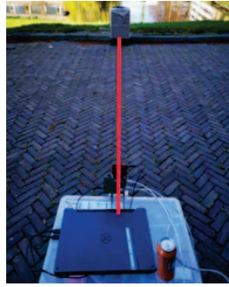
(b) Experimental setup for radome design, the radar has a front aluminum plate.
