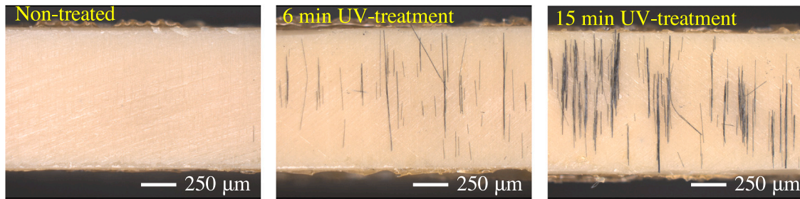
Fig. 5. Failure surfaces of the PEEK sides of the T-joints.
