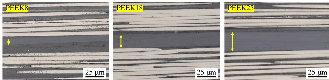
Fig. 2. Side-view images of the interleaved laminates. The yellow colour double head arrows indicate the interlayers.
