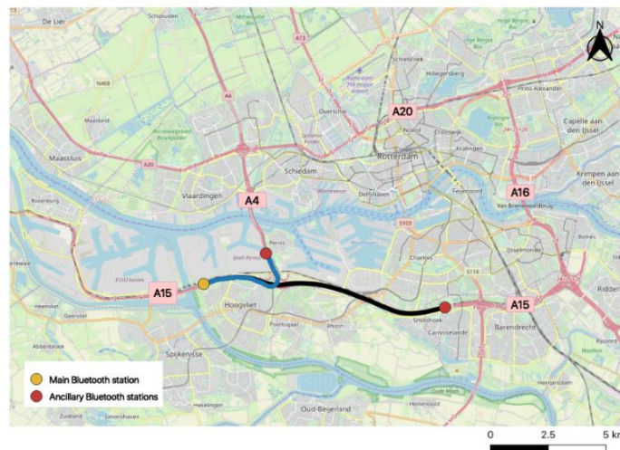
Figure 2.1. Two pairs of Bluetooth stations that can cluster travel times in both traffic directions.
