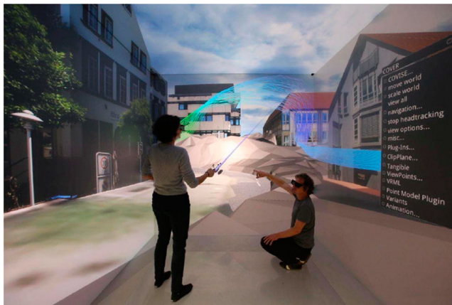
Figure 9. VR interaction with the Herremberg CDT. Particulate matter and wind flow simulation visualized in CAVE (Dembski et al. 2020).
