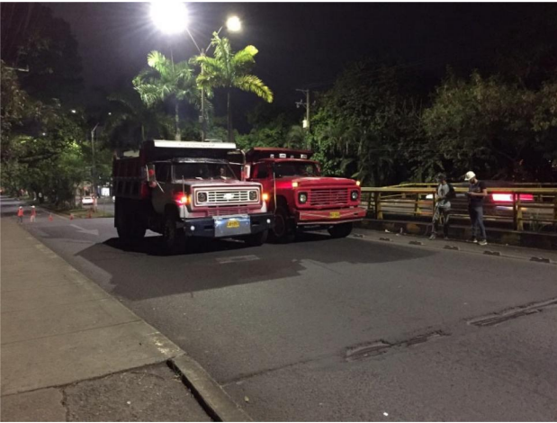
Figure 2. Diagnostic load test over the lili bridge, Cali, Colombia. For details of load test, see (Castellanos-Toro et al., 2022).
