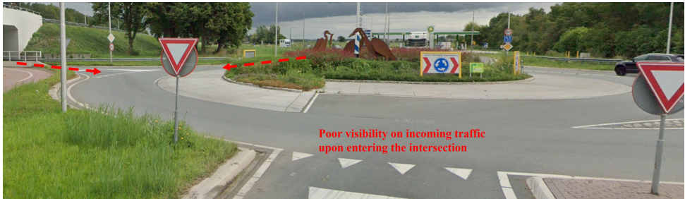
Figure 3.13: The visibility condition when entering the first roundabout on the test route. Vehicles entering from two other directions, represented by the arrows, only become visible at a distance of approximately 30 m. Image source: Google Street View
