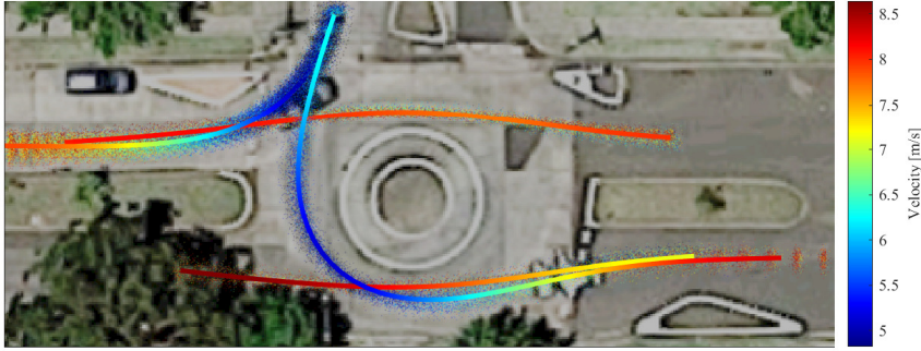
Figure 2.8: Naturalistic driving trajectories of human drivers at a roundabout. The velocity is reflected in the color map on the right. The bold lines represent the average trajectories from the same type of maneuver.
