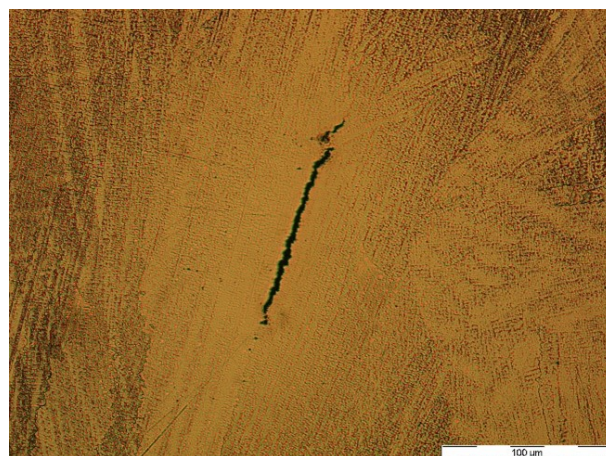
Figure 9. A micrograph of Inconel 718 showing hot cracking (liquation cracking).
