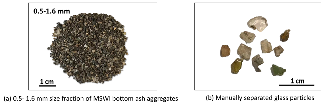
Fig. 2. (a) Image of 0.5–1.6 mm size fraction of MSWI bottom ash aggregates. (b) Image of glass particles separated from 0.5 to 1.6 mm size fraction.
