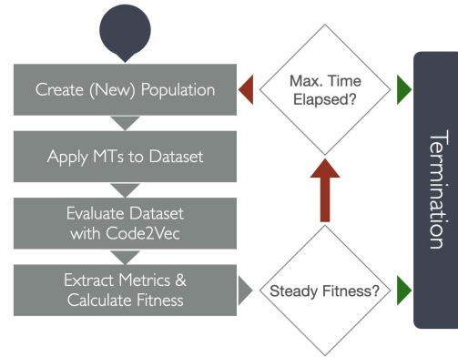
Figure 1: schematic Control-Flow of Guided-MT Program
