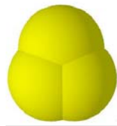
Figure 8 The Clumped-Sphere Shape Used to Model Sinter Particles
