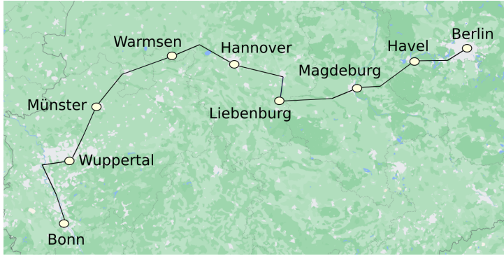
Figure 7.8: Map of Germany overlaid with a depiction of the fiber path connecting the German cities of Bonn and Berlin that we investigated. The white circles represent end nodes, in Bonn and Berlin, and repeater nodes elsewhere. This placement corresponds to the best found by our optimization method, in the sense that it allowed for minimization of hardware requirements for a target secret-key rate of 10 Hz.
