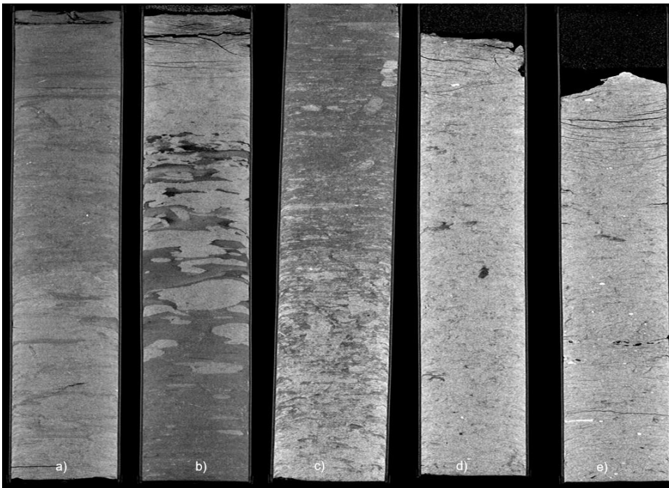
Figure 19. CT-scan images of the Paleogene Clay cores at depths (from left to right): a) 385.15-386.05 m, b) 386.05-386.95 m, c) 386.95-387.9 m, d) 387.9-388.85 m, e) 388.85-389.69 m.
