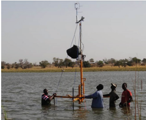
Figure 4.9: EC system installed on Lake Winkogo on a heavy-duty adjustable tripod platform
