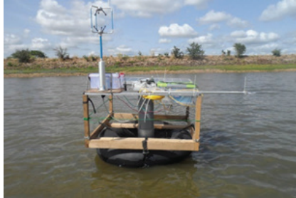
Figure 4.8: EC system installed on the 3rd floating platform in the Lake Binaba with NR Lite2 Radiometer floating on a PVC pipe fitted with an inflated rubber tube with a metal and wooden platform with the sonic anemometer at 1.90m above the water surface.
