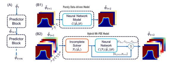
**Figure 2.** (A) Multi-step training framework helps to learn the dynamics of complete PDE solver over longer rollouts. (B1) Details of the input flow state and predictor block used in a purely data-driven approach and (B2) the hybrid NN-PDE approach, where S denotes the concatenation of different fields to obtain the complete flow state  $\tilde{\phi}$  at next time step.
