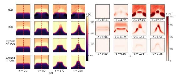
Figure 11. uniform-Bunsen case with constant inlet velocity U = 0.375 and E = 0.95. (A) Temperature field predictions; (B) Absolute error between ground truth ( $\mathcal{P}_c(T_t)$ ) and the output predicted—from top to bottom top—by: FNO, purely data-driven approach and hybrid NN-PDE. Hybrid NN-PDE model predicts physically accurate evolution of the flame cases under study.
