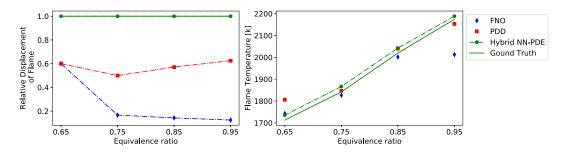
**Figure 8.** Hybrid NN-PDE approach predicts physically accurate results with correct flame temperature and relative displacement of flame front across different equivalence ratios.
