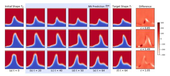
**Figure 22.** Temperature field predictions are achieved by the neural network model  $\tilde{T}_*^{NN}$  from given initial flame shape  $T_0$  to achieve target flame shape  $\tilde{T}_*$  by controlling flow velocity.
