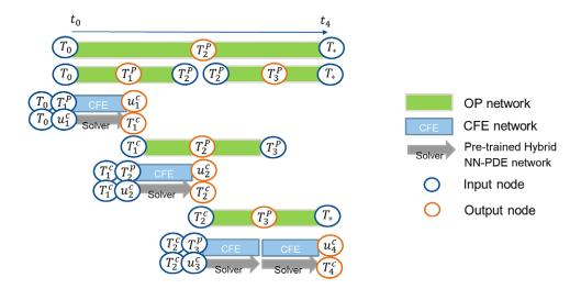
Figure 21. Details of the OP-CFE prediction sequence.
