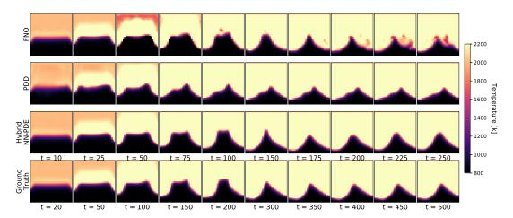
Figure 20. Comparison between different approaches at time-step  $2\Delta t_c$ —from top to bottom—FNO, PDD, hybrid NN-PDE for nonUniform-Bunsen32 test case. Hybrid approach predictions accurately match with the ground truth data over long roll-outs.
