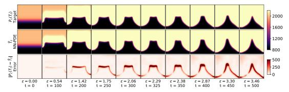
**Figure 14.** nonUniform-Bunsen100: Comparison between ground truth data  $(\mathcal{P}_c(T_t))$  and hybrid NN-PDE approach predictions  $(\tilde{T}_t)$  for a different test case of complex, high-resolution scenario.
