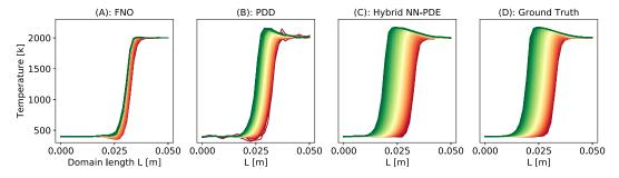
Figure 7. 1D cut of the planar flame simulation over 300 steps. The initial state is plotted in red, target state in green. Hybrid NN-PDE approach predicts physically accurate results over longer rollouts.
