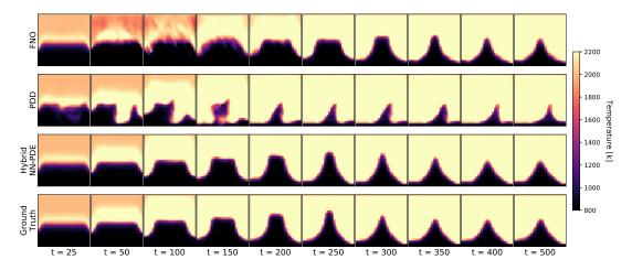
Figure 12. nonUniform-Bunsen32: Comparison between different approaches—from top to bottom—FNO, PDD, hybrid NN-PDE for a test case. Hybrid approach predictions accurately match with the ground truth data over long-rollouts of 500 time steps.
