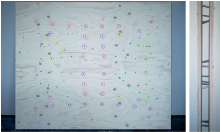
Figure 2: Favorable distribution of a specific dowel variation for the mid-section of a load-bearing wall panel (left); sideview of the specimen (right); image: Felix Schmidt-Kleespies
