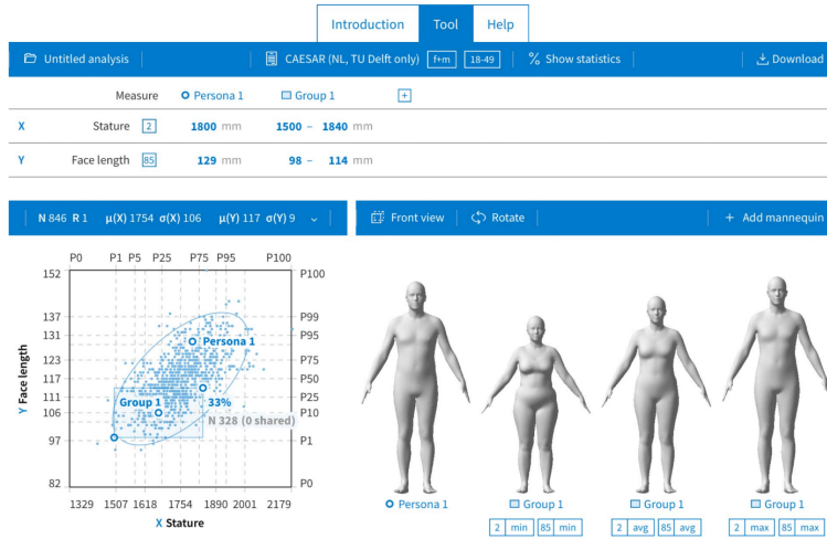
Figure 8.6: The Mannequin tool from the DINED platform [64].
