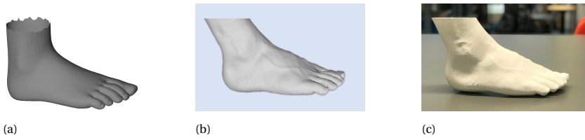
Figure 6.7: No-load foot. (a) The source mesh. (b) Scanned through Artec Eva scanner. (c) Printed Artec Eva output via Ultimaker S5 printer.
