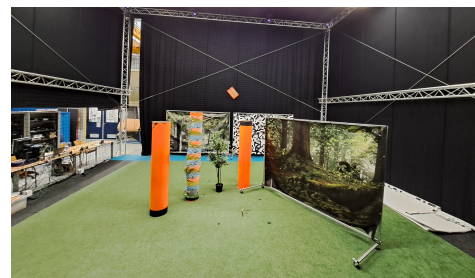
Figure 17: Real world testing environment: CyberZoo facility at the TU Delft. Obstacles are positioned to create a local minimum.
