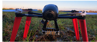
Figure 16: Experimental setup: JeVois stereo camera mounted to the bottom of the drone.
