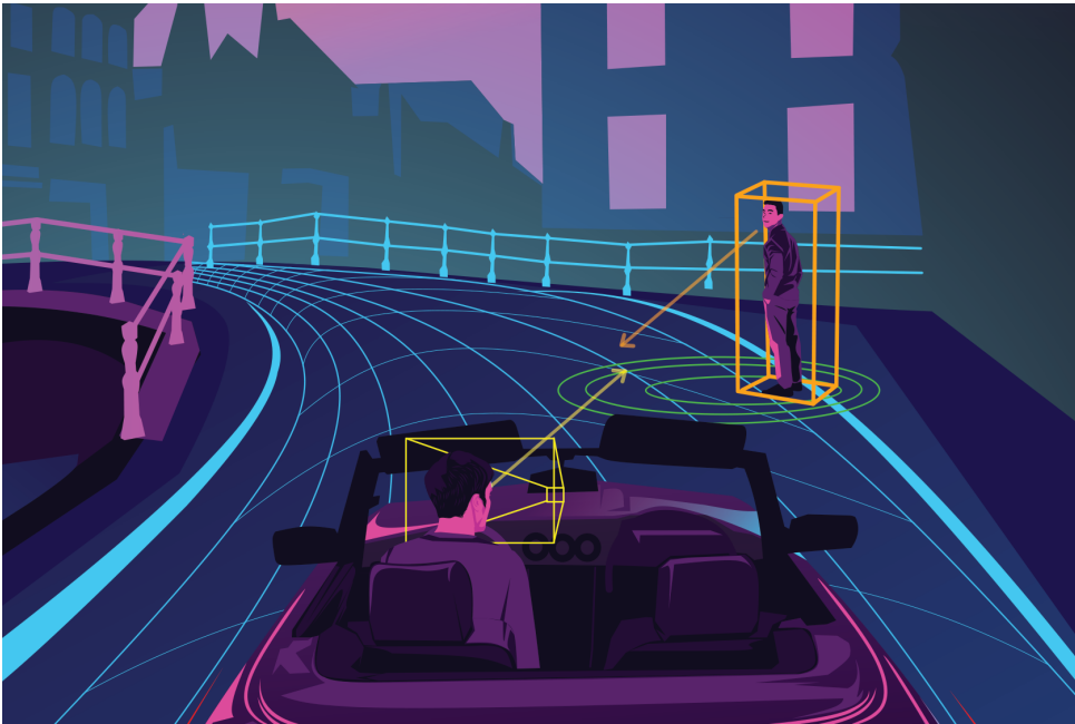
Figure 1.8: Graphical outline of the chapters of this thesis (see also thesis cover for more visual context). Chapter 3 and 4 address interior-sensing of the ego-vehicle, specifically a driver head pose dataset and a 6 DOF head pose estimation method (camera frustum and driver head pose highlighted in yellow). Chapter 5 localizes the pedestrian in 3D (orange cuboid) based on exterior camera and lidar. Chapter 6 predicts paths of ego-vehicle (blue curves) and pedestrian (green uncertainty ellipses) based on driver head pose (yellow arrow), pedestrian location (orange cuboid) and pedestrian head pose (orange arrow).
