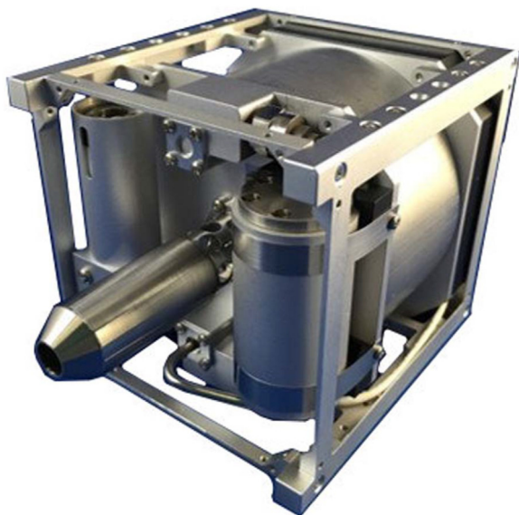
Figure 18.7 The BGT-X5 mono-propellant system from Busek [7].
