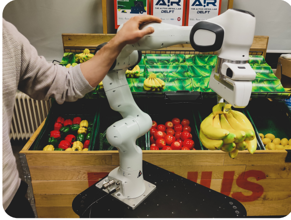
Figure 4.1: Manipulation of delicate items in a human-shared store environment.
