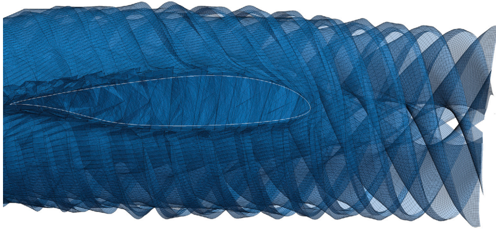
(a) Free wake results. Wake filaments penetrating through wing.
