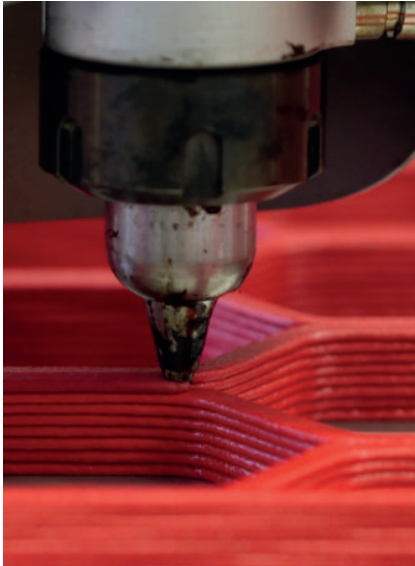
Fig. 7A: 3D-printing process of the polymer core
