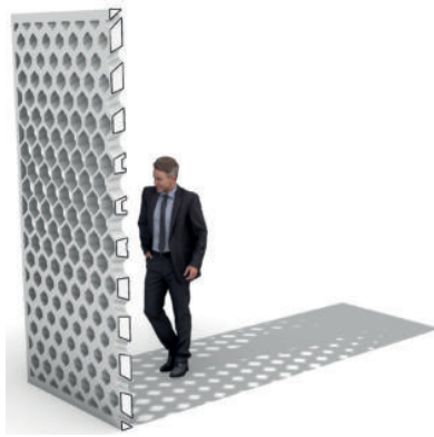
Fig 2: Rendering of a composite thin glass façade panel with 3D-printed core structure.
