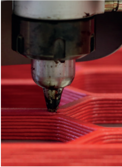
Fig. 7A: 3D-printing process of the polymer core
