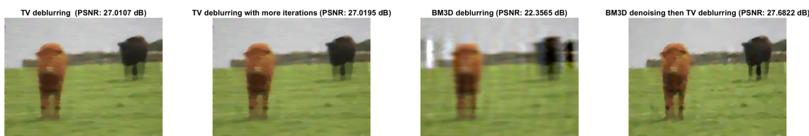
Figure 19. Typical deblurred output for the TV-based deblurrings, BM3D deblurring, and BM3D denoising followed by TV deblurring.
