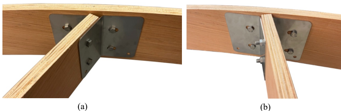
Figure 10. Second version of the connection system (a) Type 60^\circ and (b) Type 108^\circ on prototype scale.
