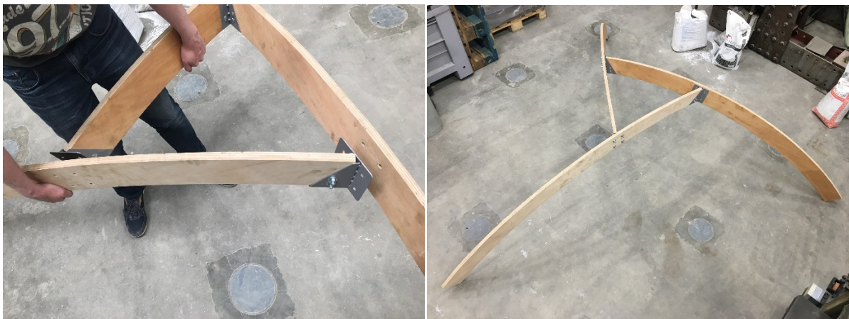
Figure 16. Assembly of a triangular fragment of the dome with the first prototypes of the Type 60° connection system and single-layer curved beams.
