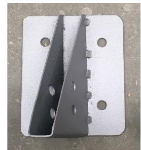
Figure 8. First version of the connection system Type 60^\circ on prototype scale.
