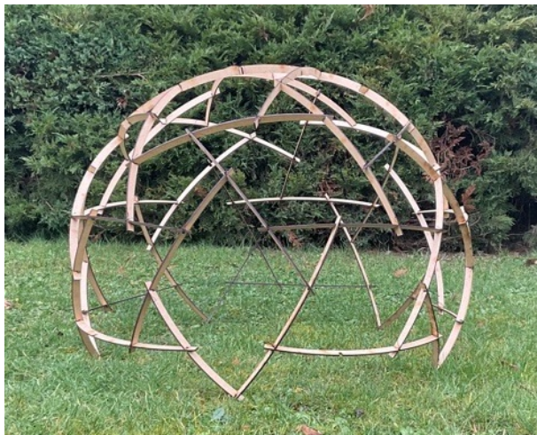
Figure 2. Model of ReciPlyDome with incisions to eliminate eccentricities and fix the structure.
