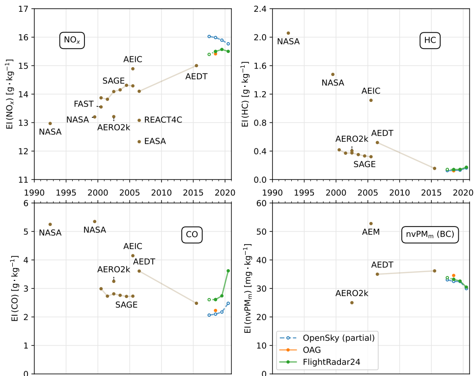
Figure 3.4: Average emission indices of NO x , HC, CO, and nvPM m in the period 2017–2020 calculated: OpenSky (partial spatial coverage), OAG, and Flightradar24. Previous estimates are shown next to the name of the institution that performed the study or name of the model used: NASA [247, 248], FAST [234], AERO2k [235], SAGE [250], AEIC [41], REACT4C [31], EASA [254], AEDT [211, 252], and AEM [232].
