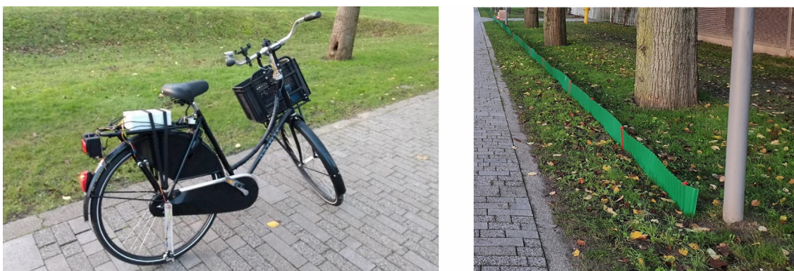
Fig. 4. The instrumented bicycle used for the experiment (left) and barrier for measuring lateral position by LIDAR (right).
