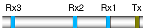
Figure 10. Illustration of an induction tool with a single transmitter and three receivers. Tx and Rx stand for transmitter and receiver, respectively.
