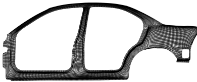
(a) Mesh of the geometry stored in car.off . The mesh consists of 31086 edges, 15895 vertices, and 62172 faces.
