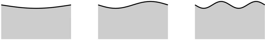
Figure 2.16: Three sine waves with the same amplitude, from left to right: \zeta(x) = -\zeta_0 \sin(ax) , a = 1, 2, 4 , x \in [0, 1] , \zeta_0 = 1/20 , supported by a foundation (gray).
