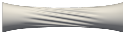
(a) Side view of the deformed annulus using the Kirchhoff-Love shell model.
