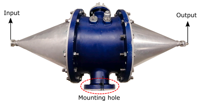
Fig. 4. Matched test bench used for sensors' characterisation.
