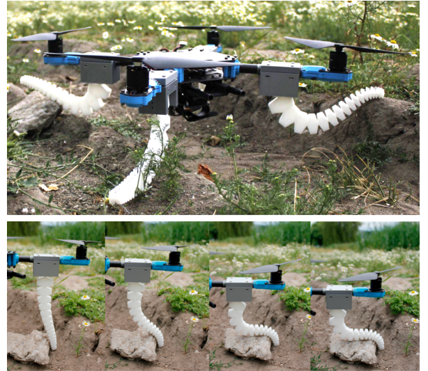
Figure 1: A conventional quadrotor equipped with passively deforming landing gear demonstrates the ability to comply with uneven terrain allowing the main body to maintain a vertical attitude. Each of the four landing arms adjusts the shape to match the environment by deforming passively according to the external forces.
