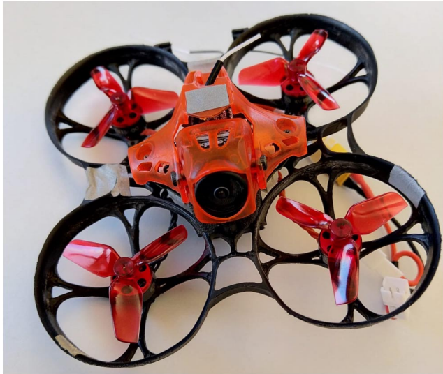
Fig. 1 The black-box-equipped 75 mm, 56 g Tiny Whoop used during experiments.
