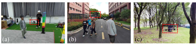
Fig. 15. Testing scenarios for obstacle avoidance. (a) and (b) are dynamic environments. (c) is a static environment. Red rectangles outline the quadrotor.
