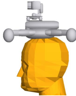
Figure 3. Scenario A impact at center of gravity of human head, i.e. \Delta = (0,0)
