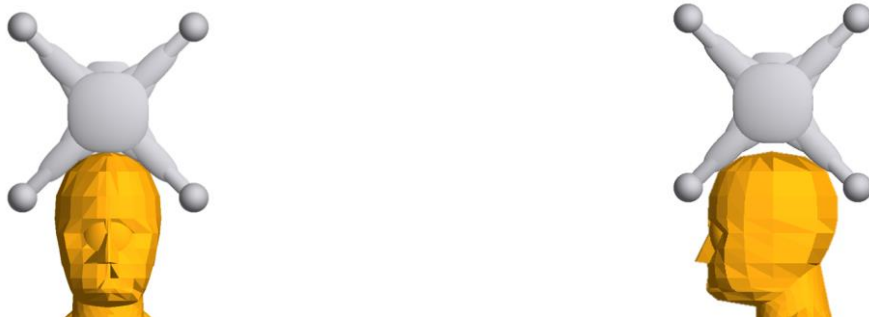
a. \theta_{roll} = 0^{\circ} , resulted P\{F|\Delta, v, \theta, \varphi\} = 92.9\% b. \theta_{roll} = 90^{\circ} , resulted P\{F|\Delta, v, \theta, \varphi\} = 23.5\% Figure 8. Examples of energy absorption by UAS arms for combinations of pitch and roll of UAS at descent angle \psi = 90^{\circ} (scenario A), pitch \theta_{pitch} = 90^{\circ} and no offset, i.e. \Delta = (0,0)
