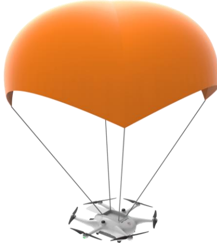
Figure 2. RA3 UAS with parachute deployed.
