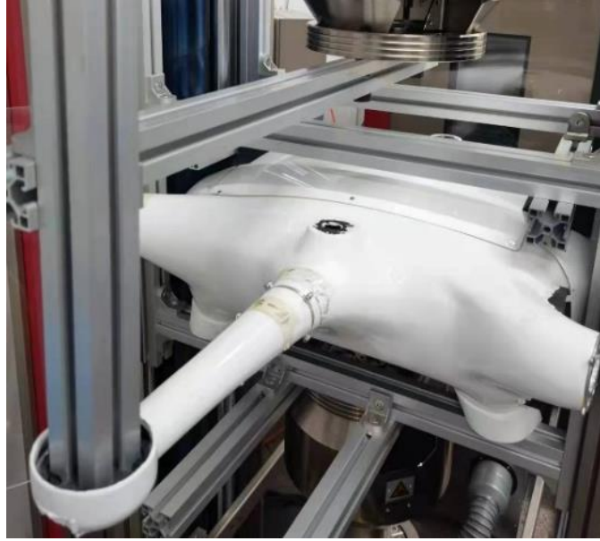
Figure A2. Quasi-static compression test of an arm of RA3 UAS
