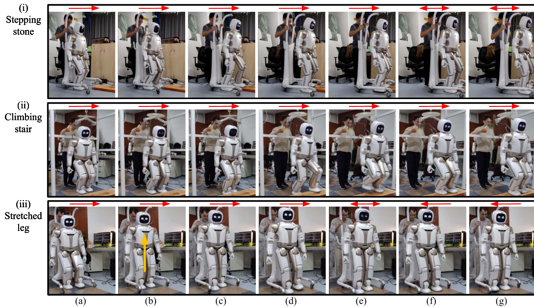
Fig. 12. Walker2 walks safely in real-world scenarios. The first , second , and third rows showcase the applications to stone stepping, stair climbing, and aperiodic walking with stretched legs. The red arrows above each row indicate walking directions and the orange arrow in (iv)(b) indicates leg stretching.
