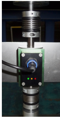
Figure 6.3: Rotary encoder / torque sensor installed on PitchVAWT
