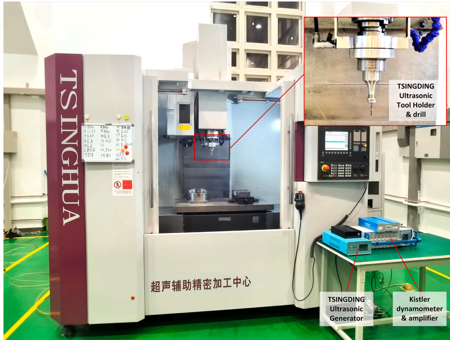
Fig. 3. Schematic presentation of Machine setup for drilling tests [37].
