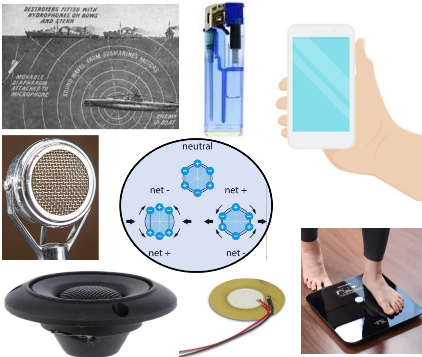
Figure 1.1: Piezoelectric elements in everyday life. Piezoelectric element in middle is shown as a crystal structure with equal amount of positively and negatively charged atoms. When applying pressure (left atom schematic) a net charge appears on the surface and reversing this has the inverse effect (right atom schematic). Examples shown starting clockwise at top-left: submarine sonar, lighter, smartphone, weight scale, electroacoustic transducer, speaker, and microphone. Figures adapted from [3–9].
