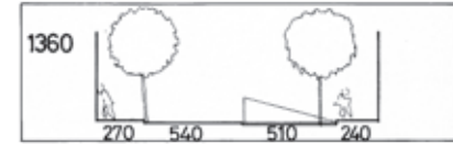
One-sided parking, perpendicular r_p = 0.4 parking lots/m ( b > 15.60\text{m} )
