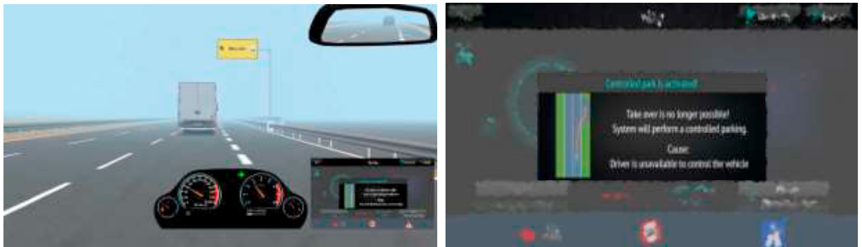
Fig. 4. (a) Critical scenario: starting an MRM to park the vehicle in a safe area; (b) MRM warning visual cue
