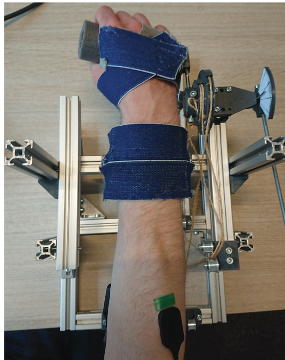
Figure 4. Top view of the setup with arm and sEMG electrodes placed on the ECR and FCR.
