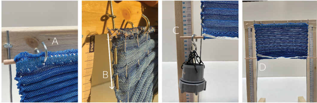
Figure 2. Textile testing setup. A) positioning on the top hooks; B) slide of the metal guide; C) progressive loading and measure of deformation; D) progressive unloading and measurement of residual deformation.
