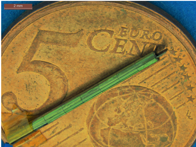
Figure 5.10: DBS demonstrator wrapped into a cylindrical probe with a length of 18 mm and a diameter of 1.2 mm on a 5 cent Euro coin.
