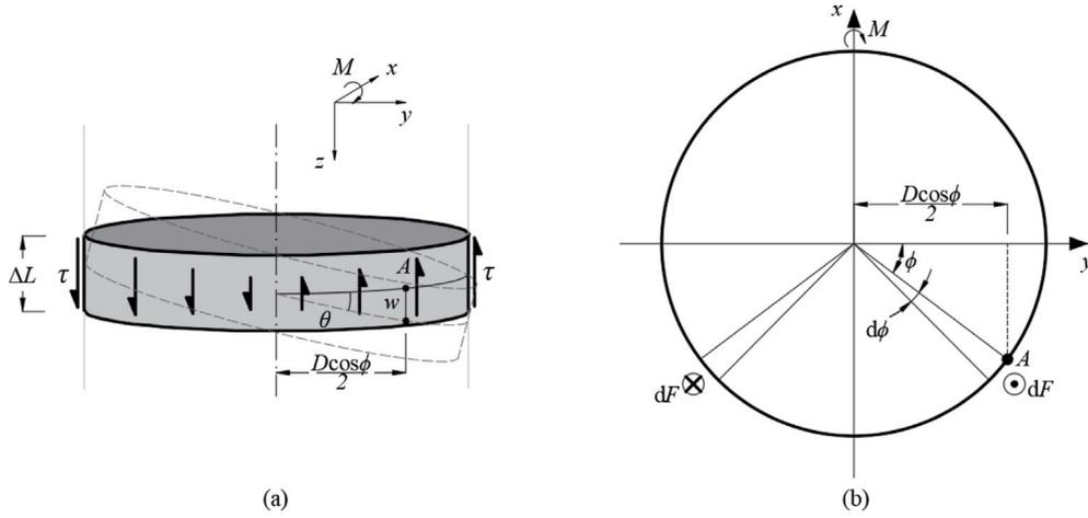
Fig. 3. (a) section side view under rotation (b) section plan view with varying shear force.
