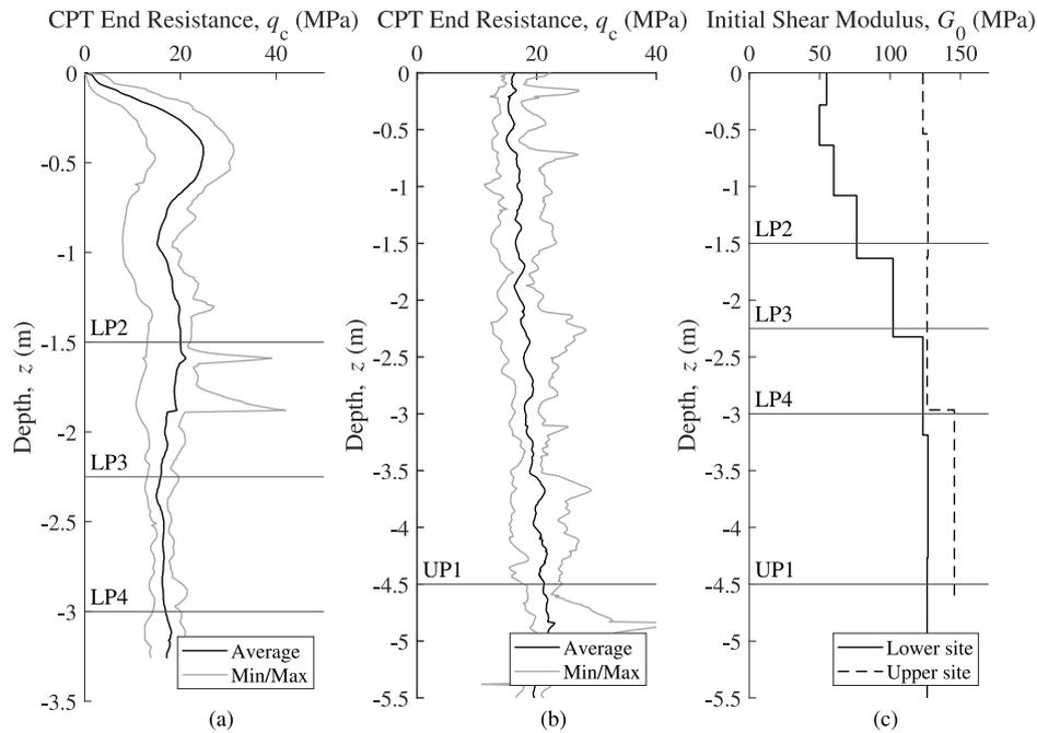
Fig. 4. (a) minimum, maximum and average  $q_c$  profiles for Blessington Lower quarry (b) minimum, maximum and average  $q_c$  profiles for Blessington Upper quarry (c)  $G_0$  profile used for Blessington Upper and Lower quarry.
