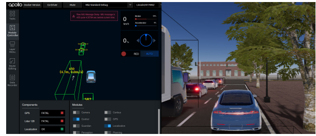
Fig. 8. Screenshot of the SVL-Apollo co-simulation, including PEM. Bounding boxes in \hat{W} are consistent between Apollo (left) and SVL (right), even undetected objects.
