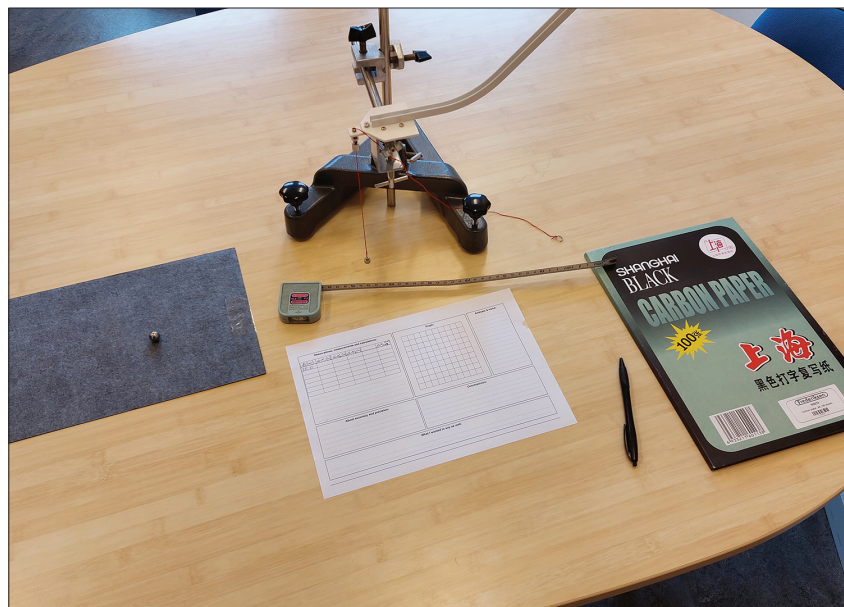
Fig. 3. The SGO is used for a horizontal projectile motion experiment.
