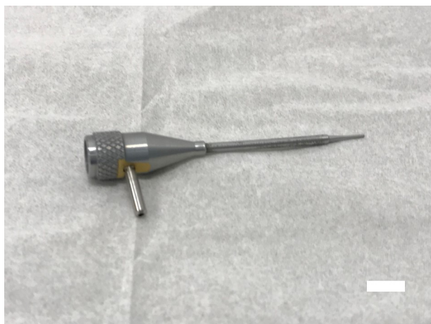
Figure 4.1: Photograph of the needle assembly with gas feed for the co-reactant. Scale bar is 6 mm.
