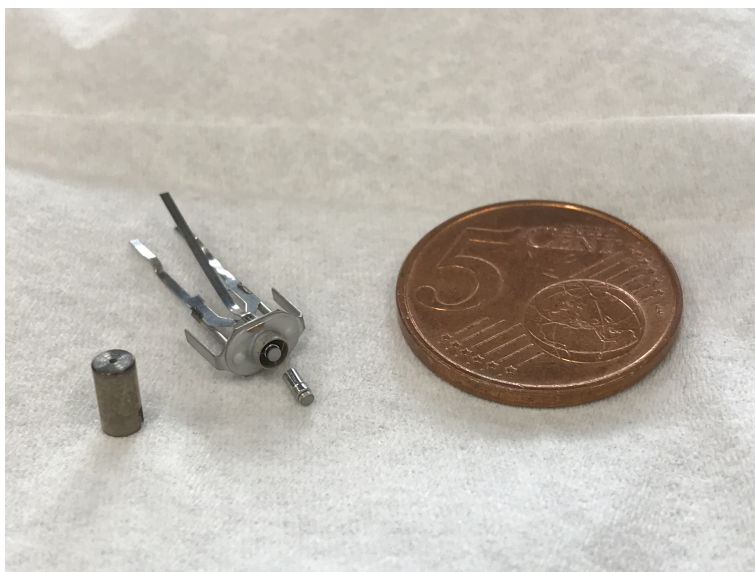
Figure 6.4: Photograph of the evaporator assembly consisting of Philips I-cathode, molybdenum cap and the heat shield with a 5 euro cent coin as a reference.
