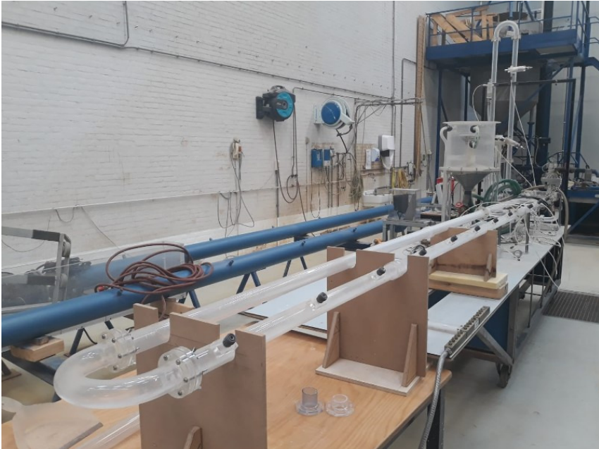
Figure 1.6: Experimental slurry loop in the Dredging Engineering laboratory at TU Delft, used for the experiments by T. Schouten. The experimental results are compared with results from interface-resolved DNS in chapter 4.
